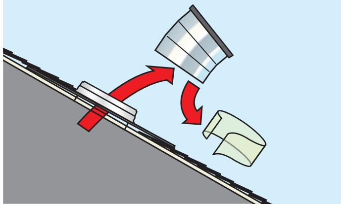
**ENGLISH:** Remove the elbow and remove protective film from upper elbow.
