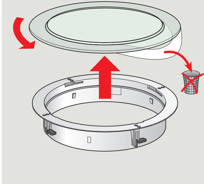
**ENGLISH:** Carefully remove the primary diffuser from the ceiling ring. Rotate the diffuser to disengage.
