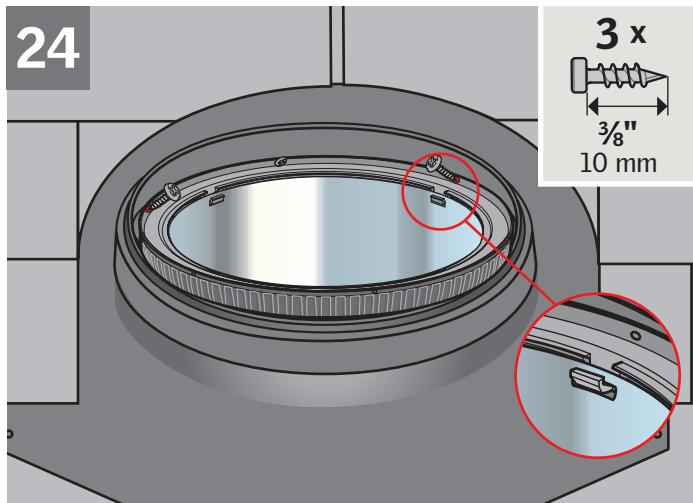
**ENGLISH:** Seat the pivot ring with the tunnel assembly into the flashing and secure with three of the 3/8" (10 mm) screws provided.
