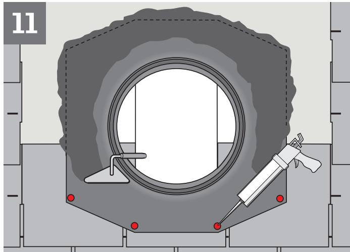
**ENGLISH:** Apply sealant as shown and seal all fasteners.
