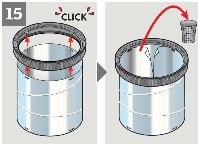
**ENGLISH:** Attach the upper elbow to the pivot ring. Make sure all pivot ring tabs engage with a click. Remove protective film from the upper elbow.
