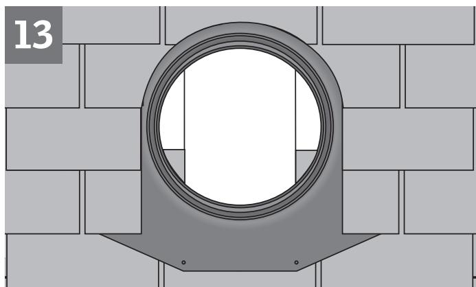
**ENGLISH:** Reinstall roofing material over the flange. Leave a  $\frac{5}{8}$ " (15 mm) channel for water to run off.
