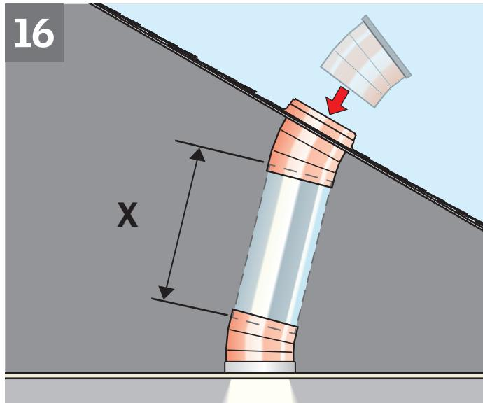
**ENGLISH:** Adjust the angle of the upper elbow so that it points directly against the lower elbow. Elbows can be damaged if excess force is applied.
