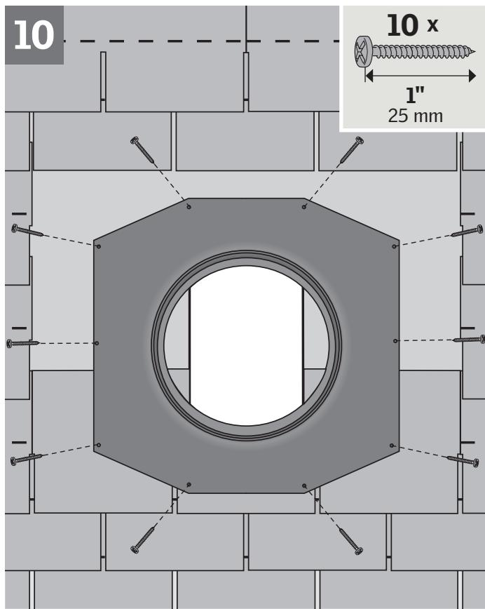
**ENGLISH:** Center the flashing over the rough opening and secure the flange with screws in all the pre-punched holes along the edges.
