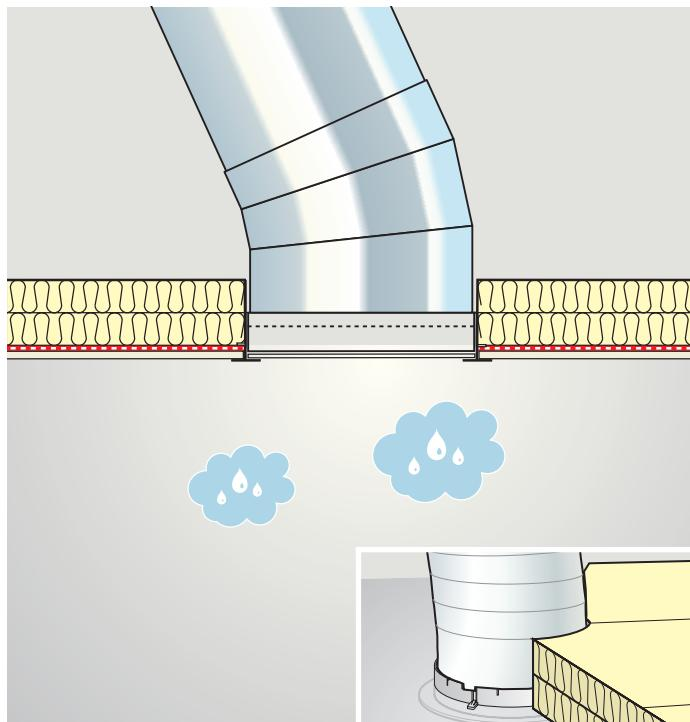
**ENGLISH:** Install the diffuser assembly by aligning the notches and rotate to secure.
