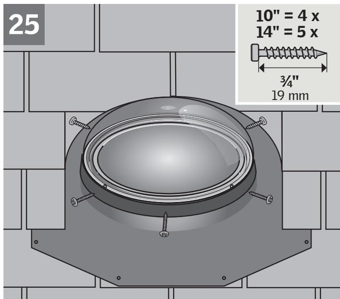
**ENGLISH:** Align holes; install and secure the dome with the 3/4" (19 mm) screws provided. Do not overtighten the screws.
