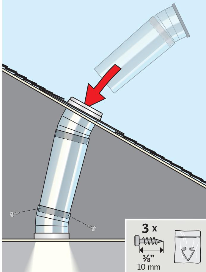
**ENGLISH:** Connect tunnel assembly with the clips supplied. If tunnel section was trimmed or holes do not align, use the screws supplied as necessary.
