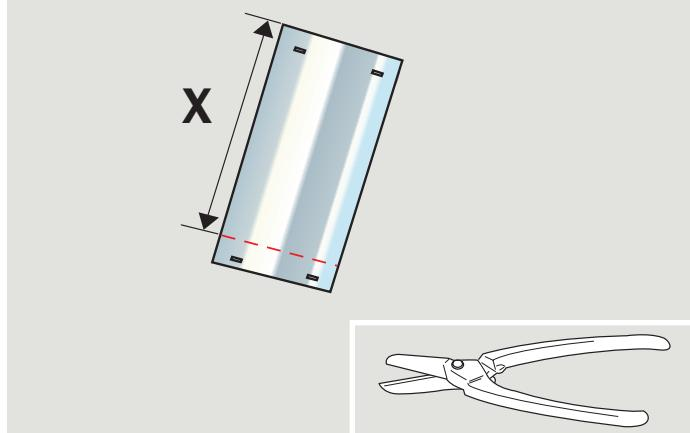
**ENGLISH:** With one rigid tunnel section, cut the section to length.
