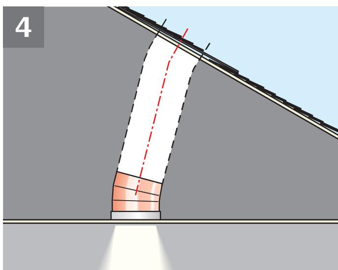
**ENGLISH:** Adjust the angle of the lower elbow. When it is positioned correctly, it will be in line with the upper elbow. Elbows can be damaged if excess force is applied. Refer to the illustration for optimal positioning.
